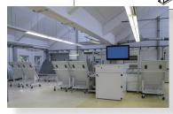
Fully automatic sorting according to print job into 6 stacker bins. A slip sheet is inserted after each plate. Additional routing papers are printed for each job. The contents of the plate cart is shown on a 50" monitor.
