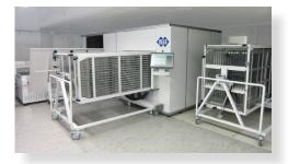
LogiStack plate storage with pivoting plate cart for transport of plates to the press. The plates are inserted horizontally into the cart (left), then the plate magazine is pivoted and the plates are brought hanging to the press (right).
