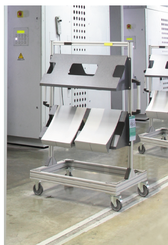
Plate trolleys for the supply of plates to the lower press units.
