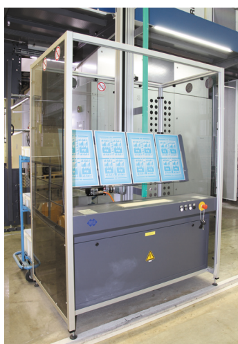
Pre-sorted plate sets for multiple press units can be transported simultaneously.
