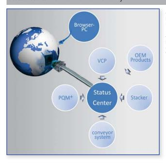
All components of a plate processing line may be integrated in the NELAStatusCenter. An internet interface provides access through any Internet or Intranet workstation.
